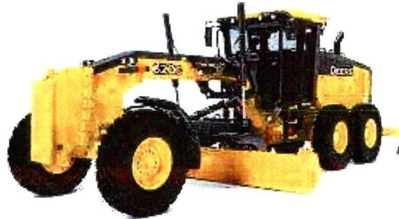
**MOTONIVELADORA NOVA, MARCA JOHN DEERE, MODELO 620G**
